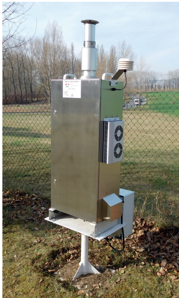
Obr. XI.6 Stanice MIM Vyškov – vzorkovač (ČHMÚ, pobočka Brno) Fig. XI.6 MIM station Vyškov – sampler (photo: CHMI, Brno Regional Office)
